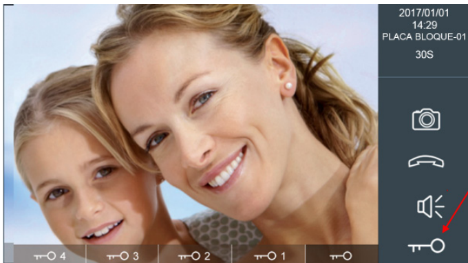
Additional electric locks activation
