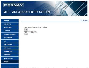
**FACTORY SETTINGS:** The panel will automatically turn off and start up with the factory settings. We refer below the essential default parameters for your reference.
