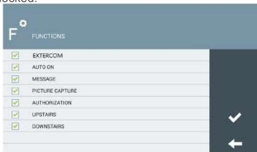
In the case of disabled functions, the corresponding icon will appear on the screen, but its use will be blocked, and a message will appear. "FUNCTION NOT ACTIVATED".
