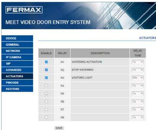
Click on ENABLE the relays to be enabled and write the name or description that should appear on the monitor when you want to control any of them.
