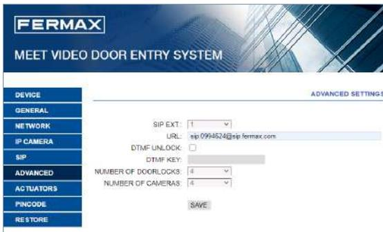
**SIP EXT.:** Use this drop-down to set up call forwarding from this monitor to other devices (NONE, 1, 2, 3 or 4). The form will be automatically adapted depending on the number chosen.
