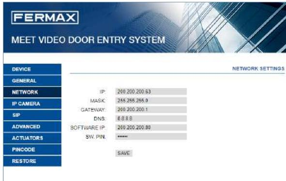
**IP:** IP address to be assigned to this monitor.
