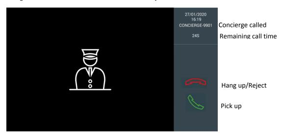
Depending on the installation, you may see an image captured by a camera installed next to the concierge
