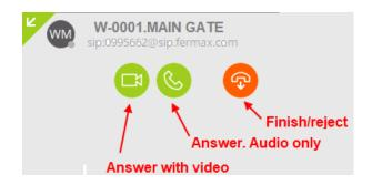
Once a call is answered (with or without audio) a new pop-up will appear with the image from the panel's camera and a panel with several function to use during the conversation (mute, hide image, speaker off, etc.).
