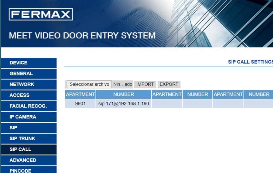
The screenshot displays the 'SIP CALL SETTINGS' configuration page for the FERMAX MEET VIDEO DOOR ENTRY SYSTEM. On the left is a vertical menu with the following items: DEVICE, GENERAL, NETWORK, ACCESS, FACIAL RECOG., IP CAMERA, SIP, SIP TRUNK, SIP CALL (highlighted), ADVANCED, and PINCODE. The main content area features a header with 'SIP CALL SETTINGS' and a toolbar with 'Seleccionar archivo', 'Nin...ado', 'IMPORT', and 'EXPORT' buttons. Below the toolbar is a table with the following data:
