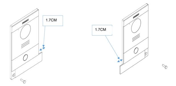
,4Move the slider of the panel and fix the two screws, when installing, pay attention to the reservation of the 1.7CM space around the door to move the slide cover.
