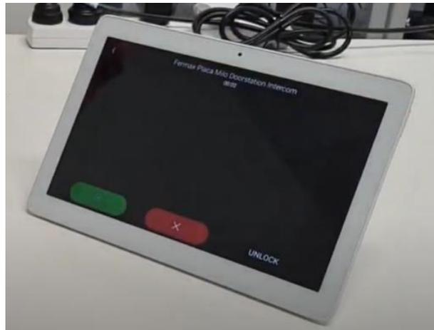
Pressing the answer button will display the video from the camera and open the bi-directional audio channel. The timing is limited to 120". You have the option of opening the door at any time.
