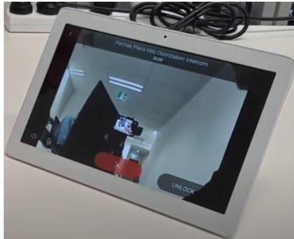
Note: the video display before going off-hook is not available because C4 does not allow this functionality via SIP protocol (video preview).
