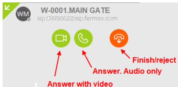
Once a call is answered (with or without audio) a new pop-up will appear with the image from the panel's camera and a panel with several functions to use during the conversation (mute, hide image, speaker off, etc.).
