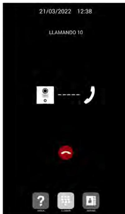
The called station will receive the ringing tone and call origin information by displaying the Tag defined on the outdoor panel and the camera image (depending on whether the receiving device has a video receiving option). The call will ring for a maximum of 30 seconds.
