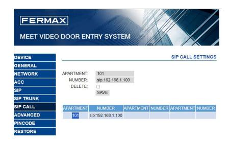
REMARK: These telephones are SIP, so they can be also registered as an extension of a SIP server. If that was the case, and assuming that the server ip would be 192.168.1.199 and the phone extension registered 1122, the call destination to be used would be then <a href="mailto:sip:1122@192.168.1.199">sip:1122@192.168.1.199</a>. Where this syntaxis corresponds to <a href="mailto:sip:sip">sip:sip</a> extension@server ip address
