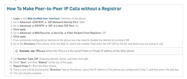
The screens where to setup the SNOM parameters are the following:
