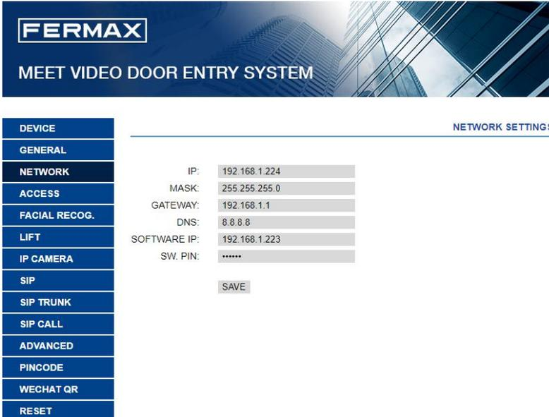
The screenshot shows the FERMAX MEET VIDEO DOOR ENTRY SYSTEM interface. On the left is a vertical menu with options: DEVICE, GENERAL, NETWORK (highlighted), ACCESS, FACIAL RECOG., LIFT, IP CAMERA, SIP, SIP TRUNK, SIP CALL, ADVANCED, PINCODE, WECHAT QR, and RESET. The main area is titled 'NETWORK SETTINGS' and contains the following configuration fields:
