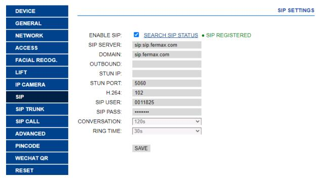
Click on SEARCH SIP STATUS to check that the board is correctly registered in the server. The SIP REGISTERED indication should appear. Otherwise, check that the data have been entered correctly and that the internet access configuration is correct.
