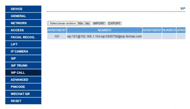
In the case of a 1L panel, the house number and the SIP address of the monitor must be configured directly and then press SAVE. The entry for that call will appear in the table.
