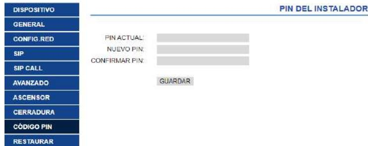
The screenshot shows a web interface for configuring the PIN. On the left is a vertical menu with the following items: DISPOSITIVO, GENERAL, CONFIG.RED, SIP, SIP CALL, AVANZADO, ASCENSOR, CERRADURA, CÓDIGO PIN (highlighted), and RESTAURAR. The main content area is titled 'PIN DEL INSTALADOR' and contains three input fields labeled 'PIN ACTUAL:', 'NUEVO PIN:', and 'CONFIRMAR PIN:'. Below these fields is a 'GUARDAR' button.
