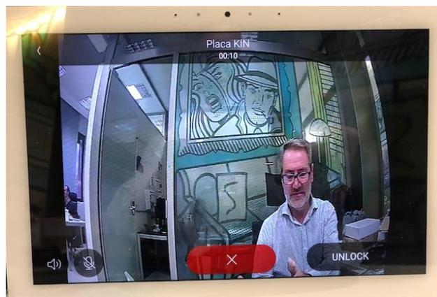
Pressing the answer button will open the bi-directional audio channel. The timing is limited to 120". You have the option of opening the door at any time. Door unlock is available pressing on the defined icon.
