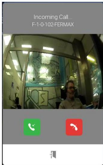
You can activate the audio or end the call. To open the door it is necessary to have previously opened the conversation.
