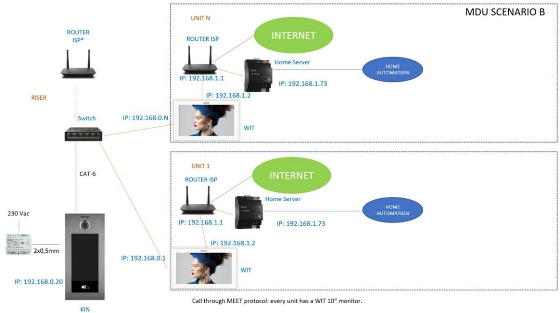
The call from the outdoor panel is secured as it does not use the internet. An internet connection is required in the building if call forwarding to the mobile is desired.
