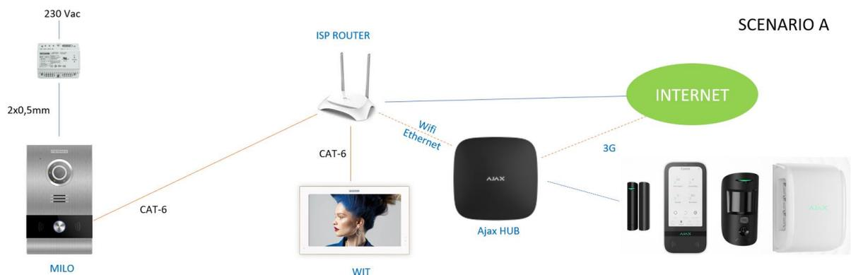
Several Meet monitors (ref. 14721 or ref.14831) can be installed, one in each room, up to a maximum of 8, with the possibility of receiving calls from the outdoor panel and also managing alarms in all of them. The RJ-45 Meet connection with static IP is used in the monitor.
